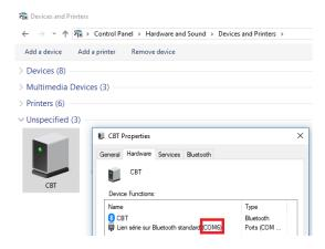
Once the interface has been paired, display the devices and connect the interface. The properties of the interface will give you the COM port number to be used on the EOBD-Facile software settings. Uncheck the "Auto detection" and select ELM327 USB when connecting.
