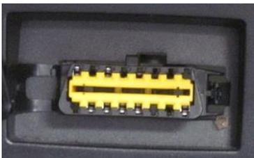
First, locate your OBD 16 channel diagnostic connector. This must be in the passenger compartment.
